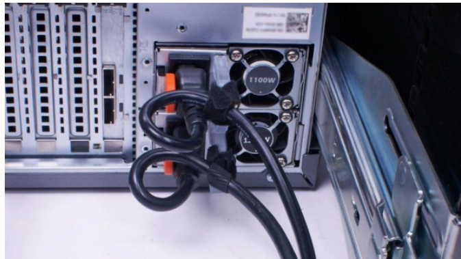
Figure 3. Routing the power cable through the strain relief on a fixed power supply
